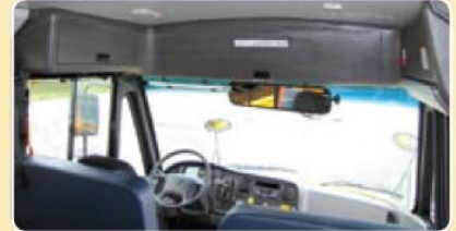
The cockpit features increased overhead storage space and improved interior rearview mirror placement.
