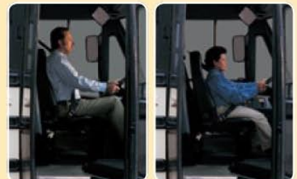
Optional tilt and telescoping steering wheel and optional adjustable pedals give drivers of all sizes the comfort they deserve.
