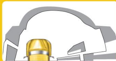
The gray area shows the 25% improved visibility over the typical Type C bus.
