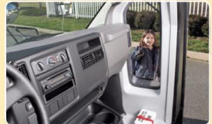
The Saf-T-Vue window offers 306 square inches of glass for optimal exterior visibility.
