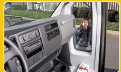
The Saf-T-Vue window offers 306 square inches of glass for optimal exterior visibility.
