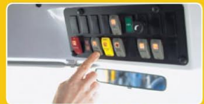
Driver switches located overhead for easy access and enhanced loading visibility.
